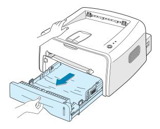
2 Remove any missfeed paper by pulling it out by the visible edge from the tray. Make sure that all of the paper is properly aligned in the tray.
